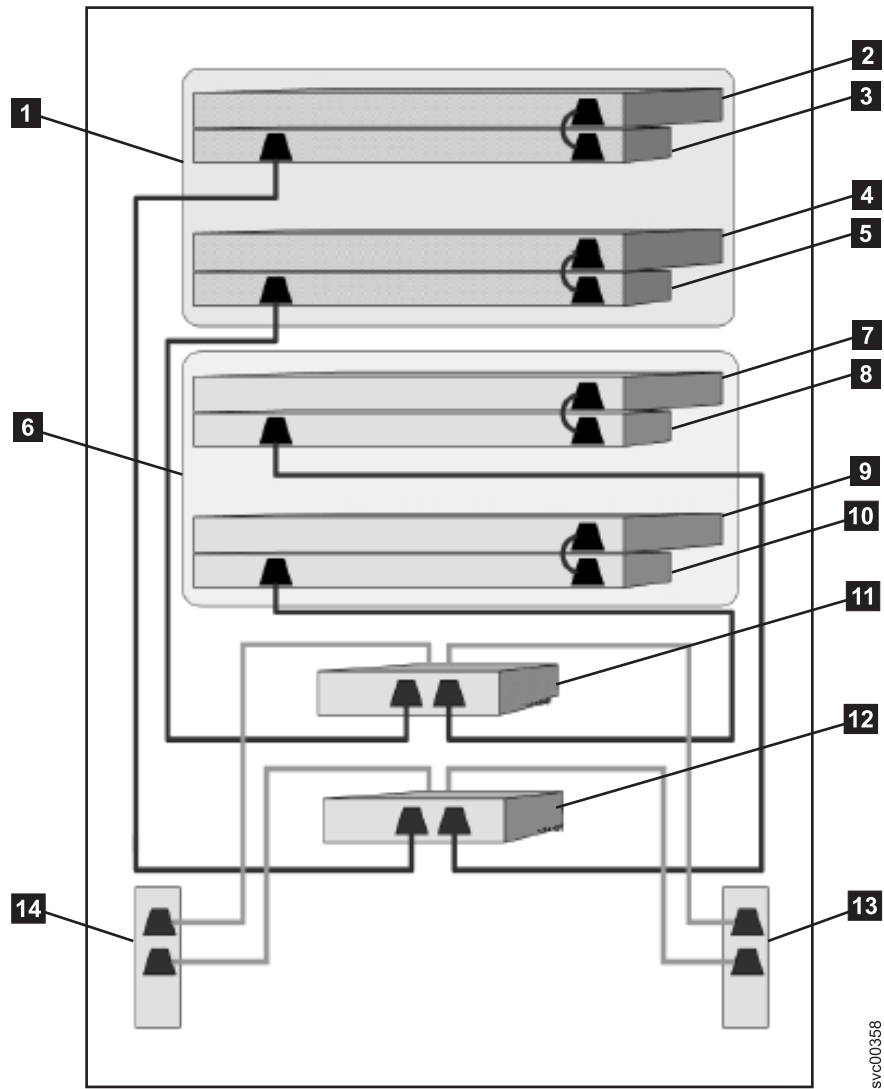
Figure 36. A four-node SAN Volume Controller cluster with the redundant ac-power switch feature
